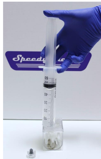
Figure 3: Inoculating a sample through the vessel port
