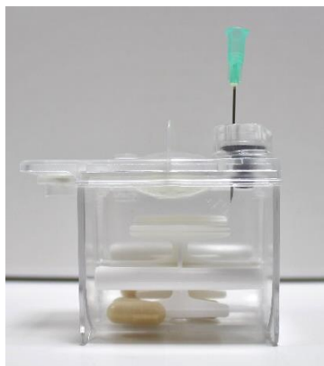
Figure 5: Pressure release needle inserted in the culture vessel.
